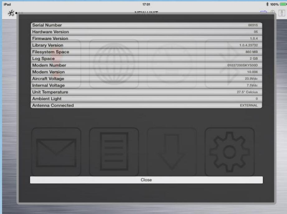
Additionally, the Aircraft Voltage (external power supply) and Internal Voltage values as well as the Unit Temperature can be used to troubleshoot any issues with the performance of the equipment.
